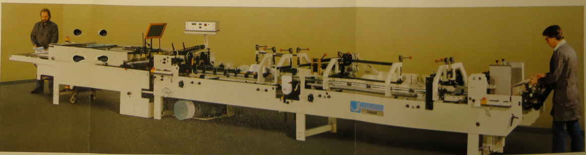
1. Feeder: easy changeover to other sizes. Feeder side walls are quickly shifted. Additional features: fine adjustment of feeder walls through micrometer screws*, vibrator* with adjustable frequency for trouble-free de-feeding of blanks, electro-magnetic clutch and brake for stopping feeder separately.
