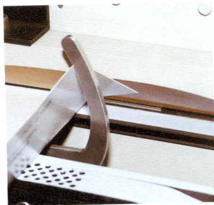
Gentle folding and high performance through special backfolding hook shape* and vacuum box* for keeping the blanks flat.
