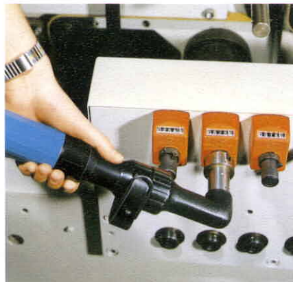
Short makeready, quick start-up and minimal start-up waste with the digital position indicator, measuring scales and compressed air motor*.
