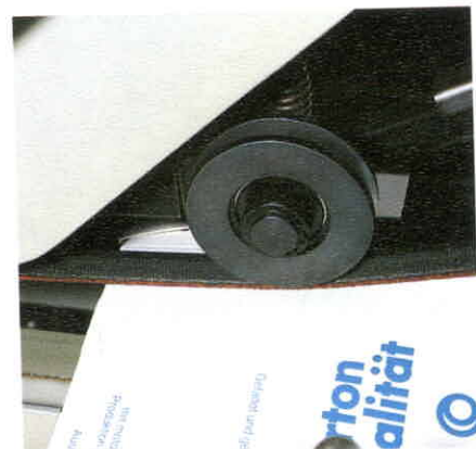
Simple adjustment and perfect folding of the most difficult lockbottom cartons with the motorized tuck-in unit*.
