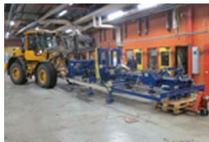
An unusual loading of the folding station to a Klett 2000 NT Inliner.
