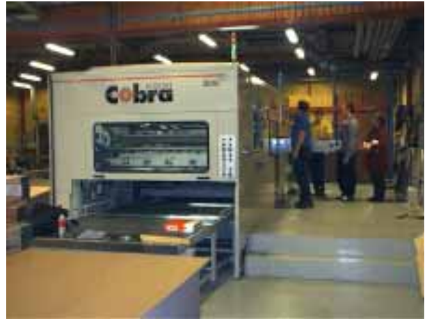
Cobra 1200 x 1620 mm flat bed die cutter with stripping and bundle stacker
