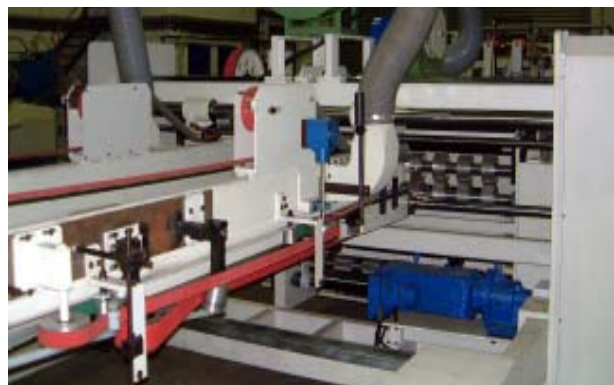
IMG ST 1228 with top print and vacuum fold station with down fold of flaps.
