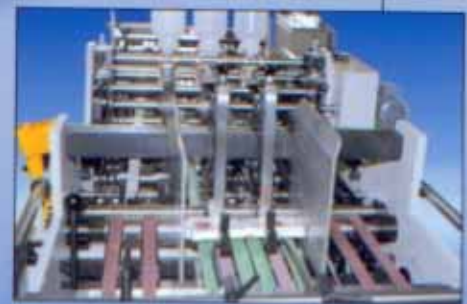
Universal timed belt feeder, movable on wheels.
