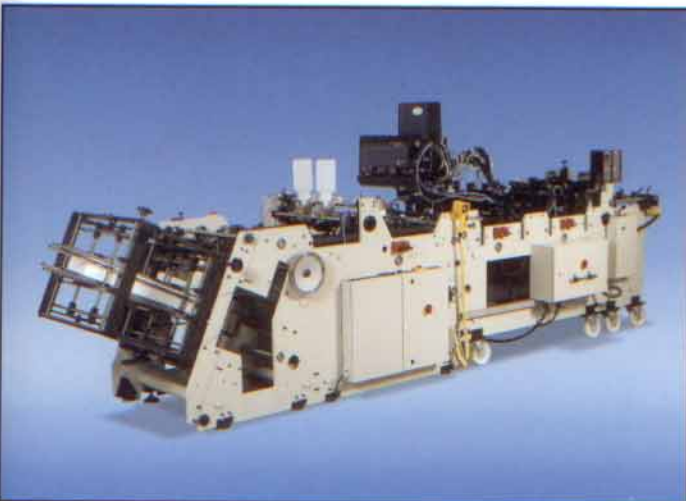
Combination of basic machine CE 650-1 with folding station for trays with two or four parallel folding flaps.
