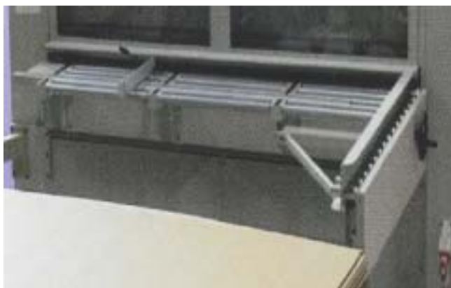
Feeder with adjustable side walls The sheets are fed in along the right side.
