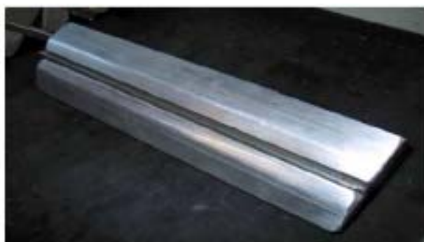
Cross creasing tool 200 mm. Saves the side lane if not all sheet width is used. Up to 2700 mm max width
