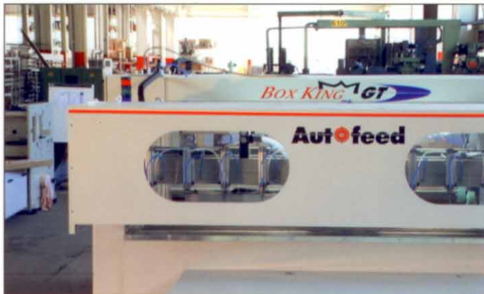
Autofeed – Automatic feeding system capable of handling any size of board in any quality (even badly warped). Comes as a system with an automatic lifting table.
