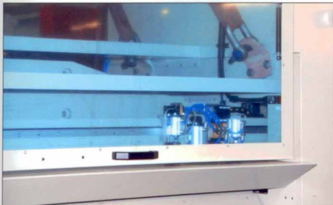
Multi tool speed slide – computer controlled cutting, creasing, scoring / perforating of the sheet in cross direction - any function from any point to any point; a substantial number of offset functions enables a great variety – patent pending
