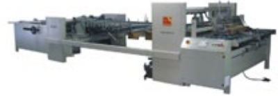
Gluers for RSC Corrugated from Inmatech, Poland
