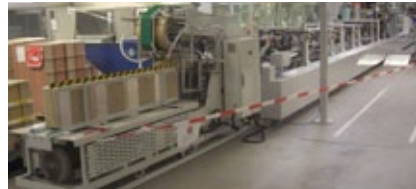
Flame sealers > 600 m/min from Gluertech, USA
