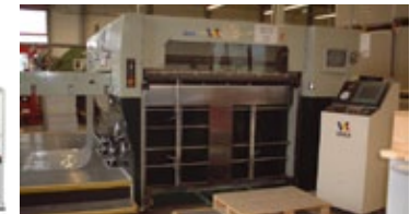
Semi automatic large flat bed die cutters from Staper/Hatten, Korea
