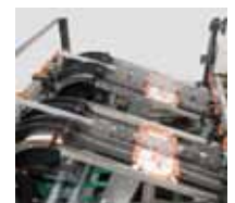
Tray types being prefolded in patented prefolder in the Gietz machine.
